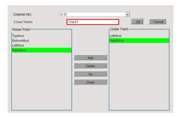
There are other buttons between the Preset points and Cruise track, you can use these buttons to adjust the order of preset points or add / delete one preset points in one cruise track.
