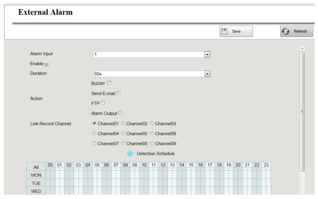
Step2 Select the Alarm Input interface from Alarm Input drop-down box list.
