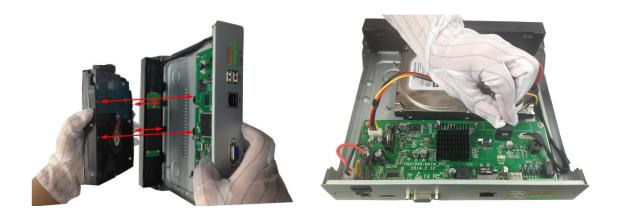
3. Place the HDD on the bottom of the device using the provided screws and then fasten the screws on the bottom to fix the HDD.
