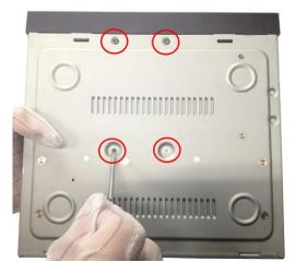
4. Re-install the cover of the NVR and fasten screws.
