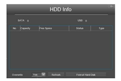
Overwrite: When the HDD is full. You can select the whether cover the earliest recording.
